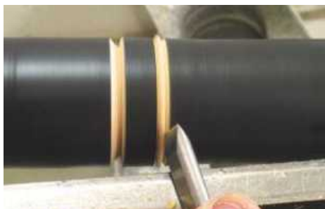
▲ Pic.16 The skew is most famously regarded as a shaping tool, especially when turning beads. Here I have cut a one-sided 'V' to mark out the position of the bead
